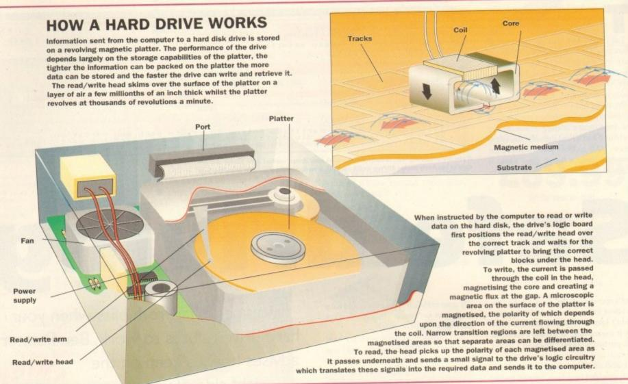
drive expert. The hard drive you have fitted to your Amiga will probably be one of two types, AT-IDE or SCSI, and these terms refer to the hardware and software that is controlling the hard drive - the hard drive "controller" - as well as the hard drive itself.
